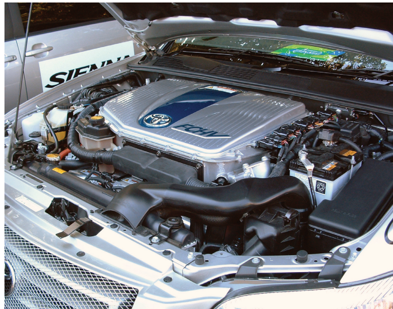
Example of a hydrogen fuel cell as used in a Toyota FCHV vehicle.
